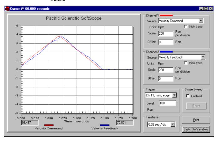
10. In the Scope window, monitor **Velocity Feedback** to see how it follows the command. Look for velocity error at speed changes. Increase **KVP** to optimize performance and miminize velocity error. If the motor starts to buzz, **KVP** is too large. Disable the drive and reduce **KVP** 20%.
