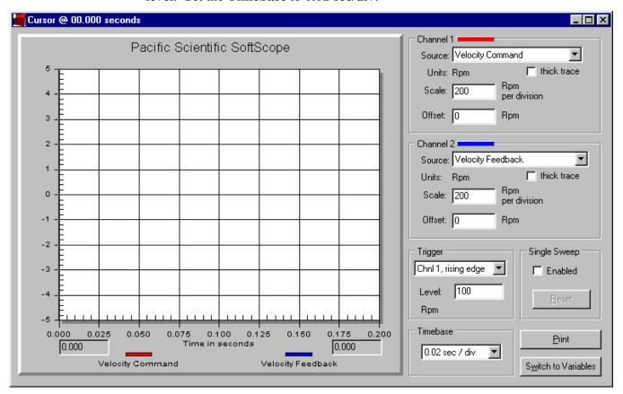
8. Use the **Switch to Variables** button to command an index move and the **Switch to Scope** button to monitor progress.
