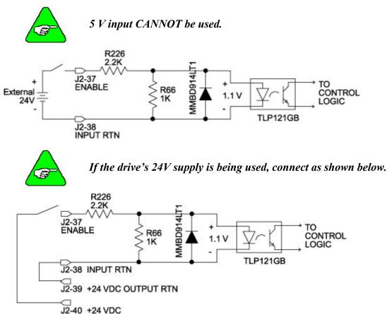
Input RTN J2-38 This terminal is the floating common return for the six optically isolated digital inputs and the optically isolated Enable input.
