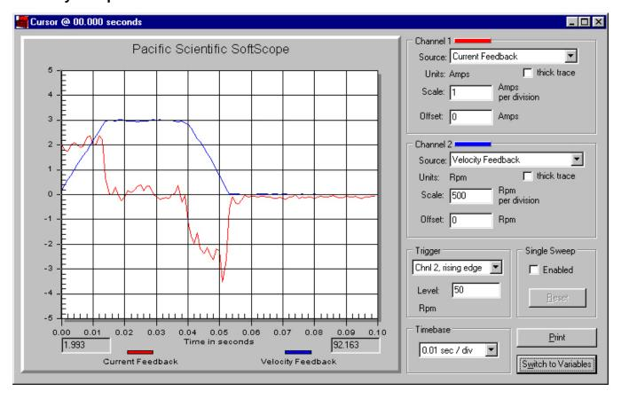
The critically-damped velocity loop follows the command without overshoot or undershoot. It has the shortest settling time and no wasted motion. Get as close to this waveform as possible.
