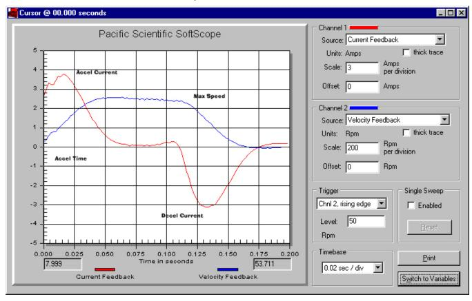
From the scope traces, record accel current, traverse current, decel current, traverse max velocity, and time to accel to traverse velocity.
