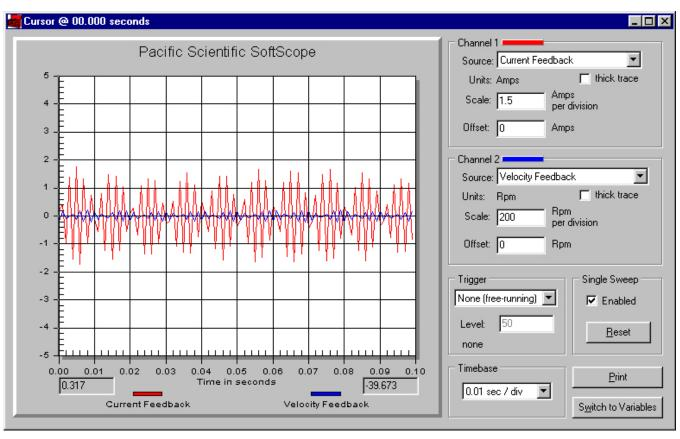
This screen capture is not a true representation of the signal waveform due to the sample resolution. However, counting the peaks over 10 divisions provides adequate results in most cases.
