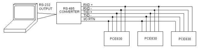
PCE830 Serial Communications Transceiver Schematic
