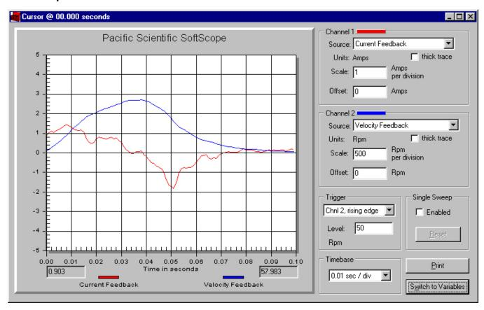
The overdamped (undershooting) velocity loop does not respond to velocity changes (disturbances) quickly. It has soft, smooth motion. It requires extra time to settle. Increasing **KVI** and/or **KVP** brings the system closer to critically-damped. Remember, when increasing **KVP**, the **ARF**x filters may need to be increased proportionally.
