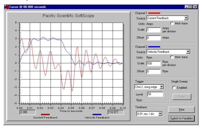
The underdamped (overshooting) velocity loop is an unstable waveform. It has wasted oscillatory motion. It requires extra time to settle. Decreasing **KVI** and/or increasing **KVP** brings the system closer to critically-damped. Remember, when increasing **KVP**, the **ARF**x filters may need to be increased proportionally. In this waveform, the oscillating current is a result of the **ARF**x filters being set too low.
