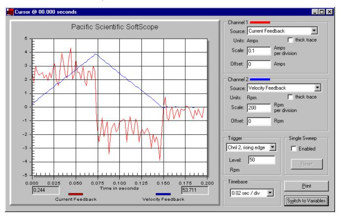
In this waveform, the current feedback is extremely low and the ripple shown is acceptable (normal) because it is much less than  $\pm$  5% of peak rated current.
