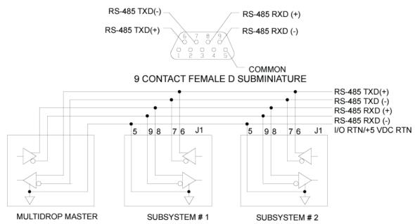
RS-232 to RS-485 Converter Installation It is often convenient to use an RS-232 to RS-485/RS-422 converter so an RS-232 port (available on all PCs) can be used to connect to multiple axes. The figure below shows a typical installation, using the B & B Model 422 RS-232 to RS-422 adapter. RS-232 to RS-485/RS-422 adapters are available from many sources.
