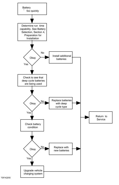
Figure 7-9. Battery Discharges Too Quickly
