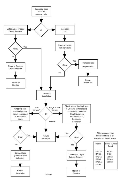
Figure 7-6. Generator Does Not Start Automatically
