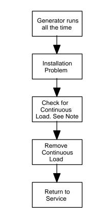
Note: Power strips with ON indicator lamps, equipment with POWER CONNECTED indicator lamps, or similar devices can place enough load on the generator to cause it to run, even though the intended load has been removed.
