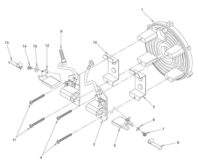
Figure 10-9: End Bell for Large Frame Generators, Earlier Version
