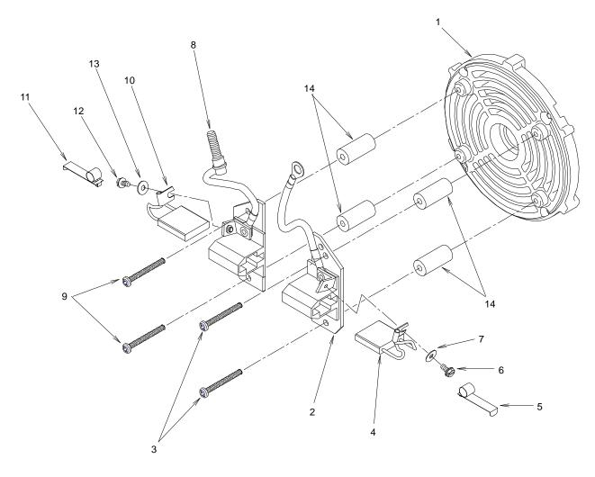
Figure 10-10: End Bell for Large Frame Generators, Current Version
