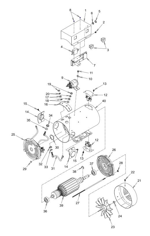
Figure 10-8: 24-Volt Large Frame Generator, Current Version, continued
