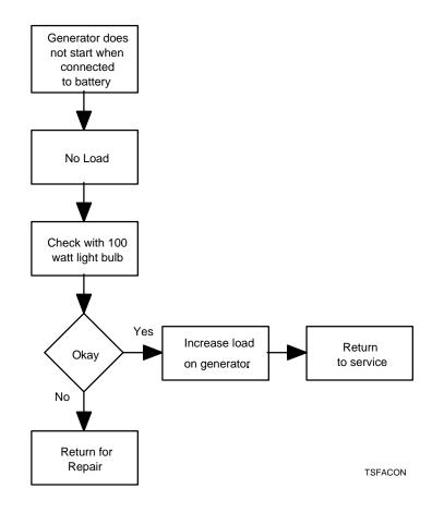
Figure 7-4. Generator Does not Start When Connected to Battery
