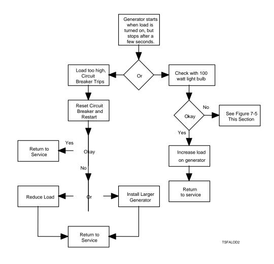
Figure 7-7. Generator Starts With Load, But Stops After A Few Seconds
