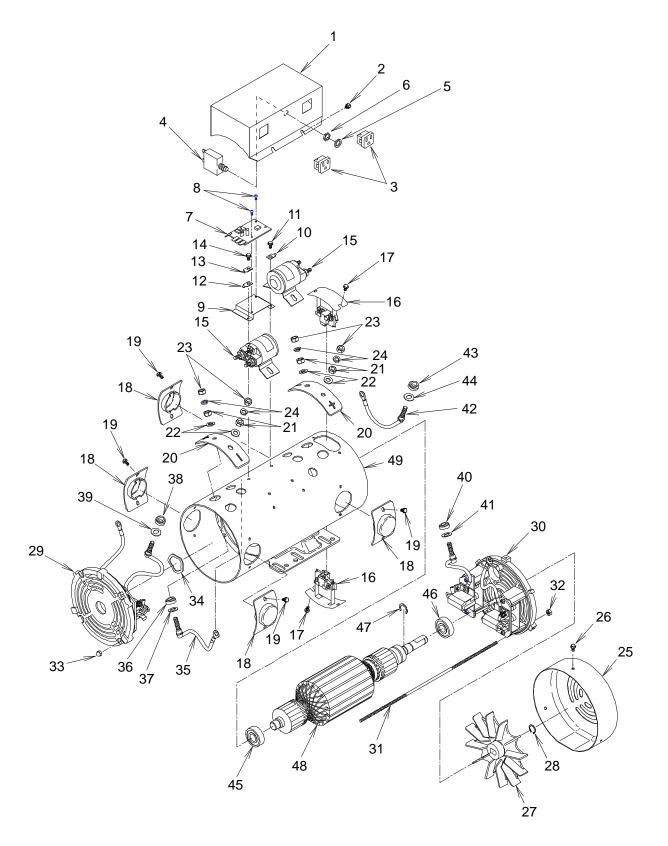
Figure 10-5: 12-Volt Large Frame Generator, Interim Version
