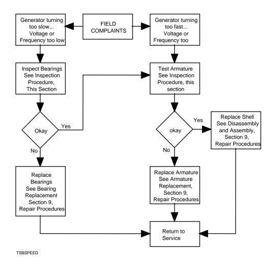
Figure 8-2. Generator Speed, Voltage, or Frequency Too High or Too Low
