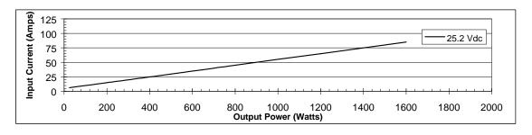
Figure 11-4: Performance Curves for DA24L-1600A Redi-Line Generators
