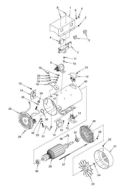
Figure 10-8: 24-Volt Large Frame Generator, Current Version
