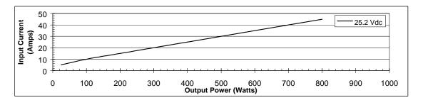
Figure 11-3: Performance Curves for DA24A-800A Redi-Line Generators
