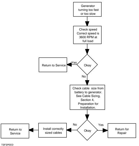
Figure 7-2: Generator Running at an Incorrect Speed
