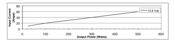
Figure 11-1: Performance Curves for DA12A-500A Redi-Line Generators
