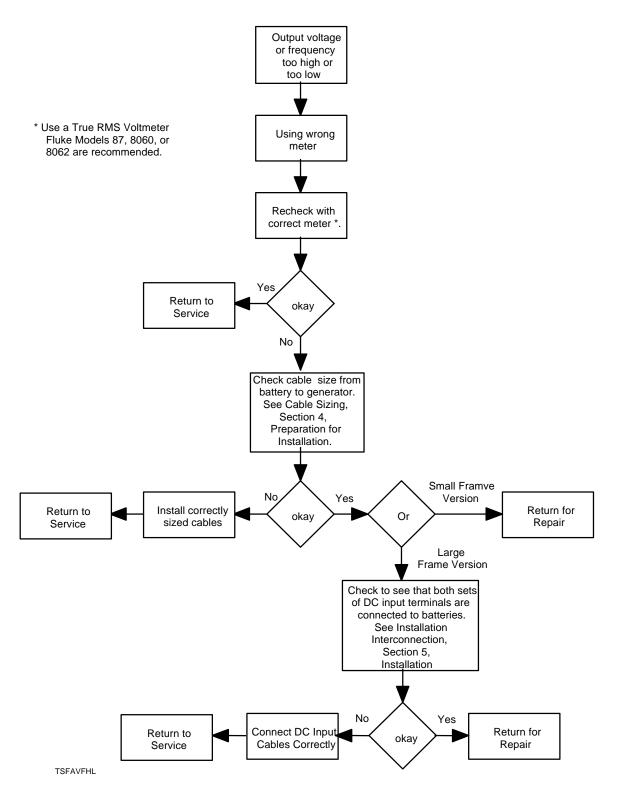
Figure 7-3: Generator Output Voltage or Frequency Incorrect
