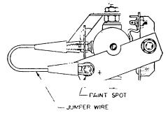
Figure 8-6. Jumper Connection - Small Frame Unit
