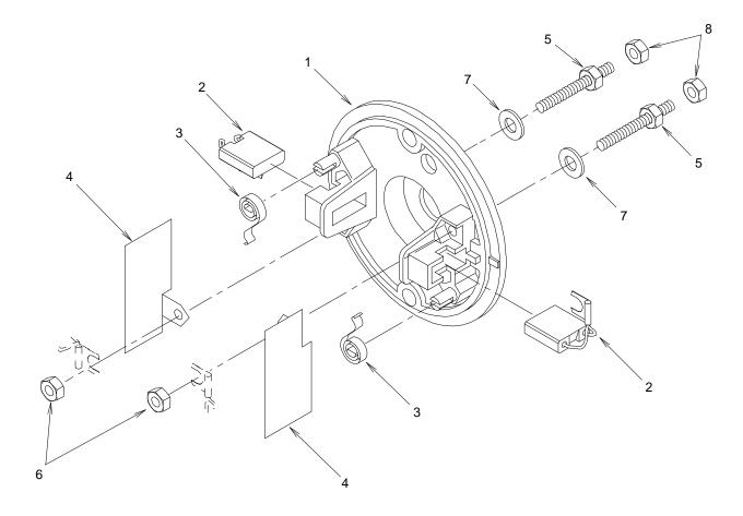
Figure 10-3. End Bell for Current Small Frame Generators
