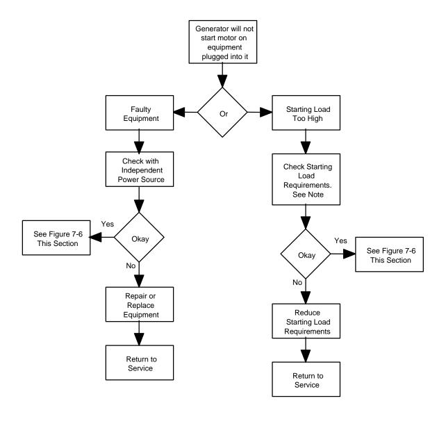
NOTE: The Redi-Line Generator can provide 1.5 its rated capacity for starting motors and loads.
