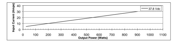
Figure 11-5: Performance Curves for DA36A-900A Redi-Line Generators
