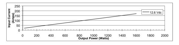
Figure 11-2: Performance Curves for DA12L-1600A Redi-Line Generators
