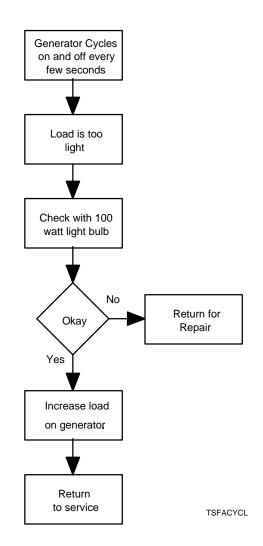
Figure 7-8. Generator Cycles On And Off Every Few Seconds
