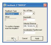
If Software Enable is active, a warning appears. The configuration change cannot be performed. Click OK on the warnings, press F12 (SW disable) and start the Feedback procedure again.
