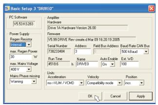
**Regen Resistor:** Change only if you use an external regen resistor. Most applications don't need an external regen resistor
