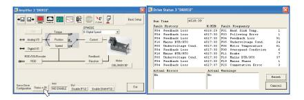
The Reset button can be used to clear some actual error messages. A description of errors/warnings can be found in the online help.
