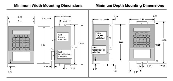
The S6961/2 depends on air flow for cooling. In all but the least demanding applications, the following mounting guidelines should be observed:
