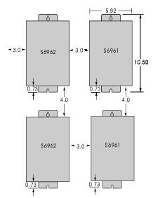
Forced air cooling may be necessary if air flow is extremely poor, if the ambient temperature is excessive (above 35(C). See *-FK1 Fan Kit*.
