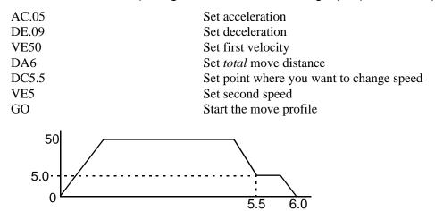
Fast In, Slow Feed Move (Using the Distance to Change (DC) command)
