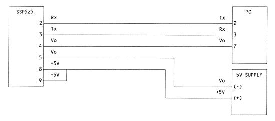
Note: Transmit (Tx), Receive (Rx) and ground (Vo) terminals on the PC may be different than labeled. Consult the the PC's owners manual for pin designations. SSP-525 Signal Common (Vo) terminals are internally connected and available on pins 1, 4 and 5. SSP-525 Power Supply input (+5V) terminals are internally connected and available on pins 8 and 9.
