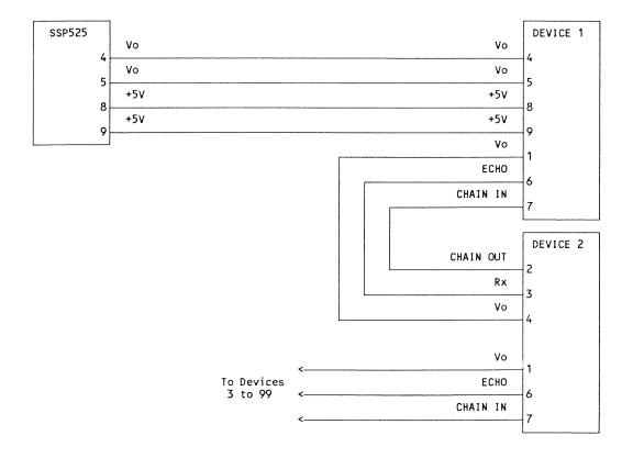
To interface the SSP-525 to a device other than a Micro Series Indexer or Direct Drive System, such as a Personal Computer or Terminal, the SSP-525 may be connected as follows:
