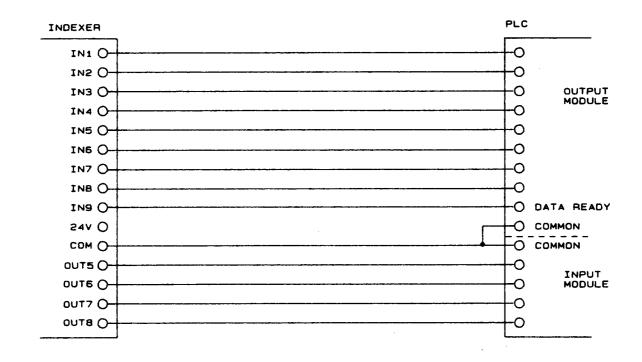
READING BCD DATA FROM A PLC USES 4 OUTPUTS AND 9 INPUTS.
