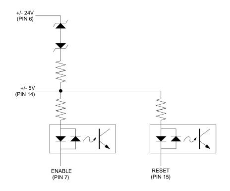
Figure 2.4 Enable and Reset
