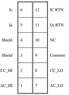
Figure 2.2. SERVOSTAR SP Series Drive Connector (C2)
