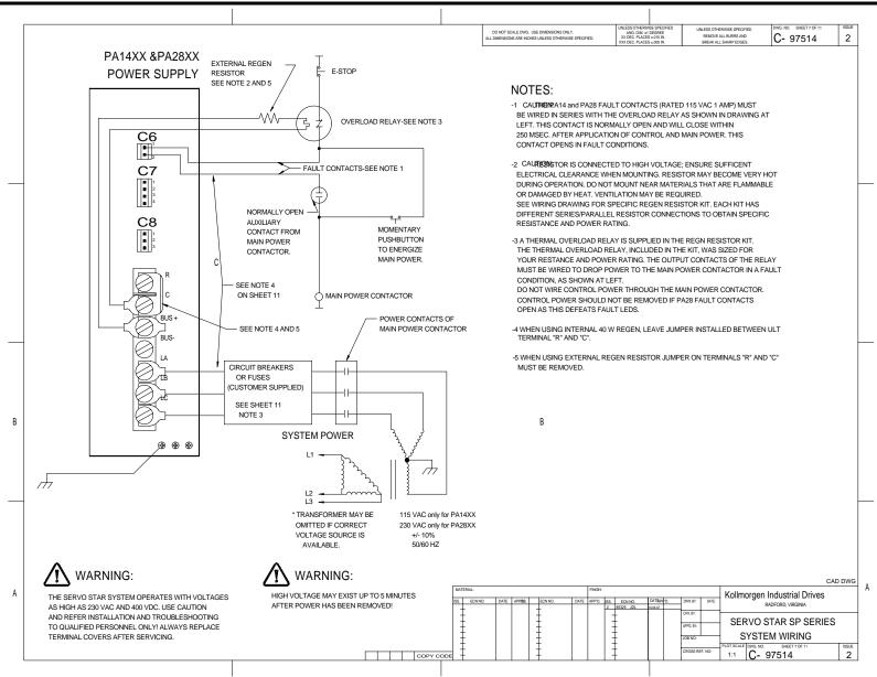
SERVOSTAR SP Series System Wiring (Sheet 7 of 11)
