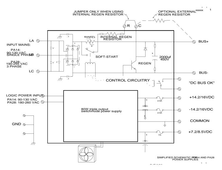
Power Supplies PA14xx and PA28xx Simplified Schematic Diagram
