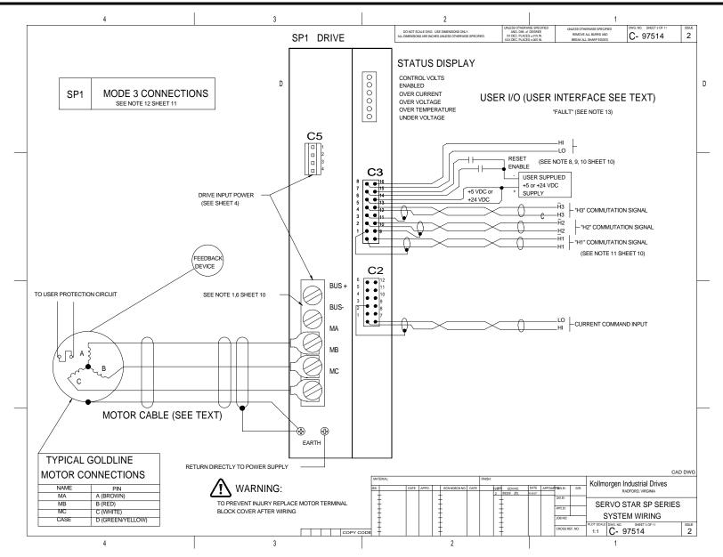
SERVOSTAR SP Series System Wiring (Sheet 3 of 11)
