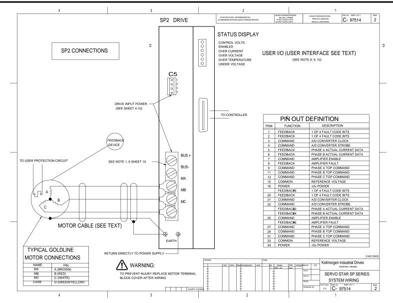
SERVOSTAR SP Series System Wiring (Sheet 4 of 11)
