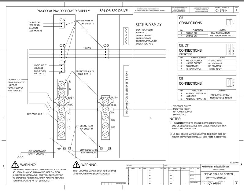
SERVOSTAR SP Series System Wiring (Sheet 6 of 11)
