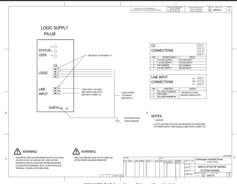
SERVOSTAR SP Series System Wiring (Sheet 10 of 11)
