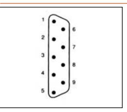
100 Series Remote Connector DE-9S Pin assignment: DB-9-S (socket, or female). Mate DB-9-P (pin or mail). Pin 1 location: upper left.
