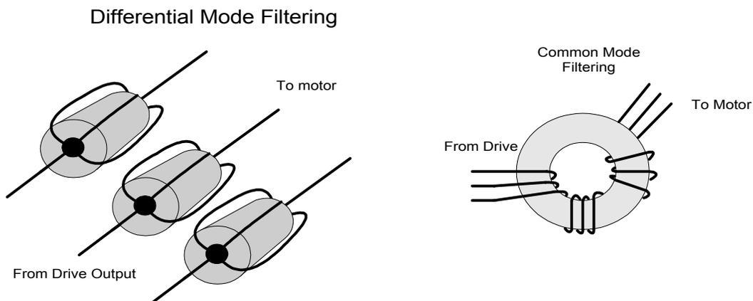
Common mode currents occur from noise spikes created by the PWM switching frequency of the drive. The use of a ferrite or iron-powder core toroid, as shown in the figure above, places common mode impedance in the line between the motor and the drive. The use of a common mode choke on the motor leads may increase signal integrity of encoder outputs and associated I/O signals. The following is a list of toroidal and ferrite cores that can be used to make common mode chokes:
