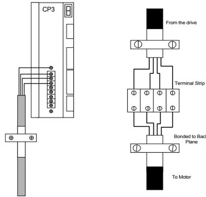
Power Block Clamp and Terminal Clamp
