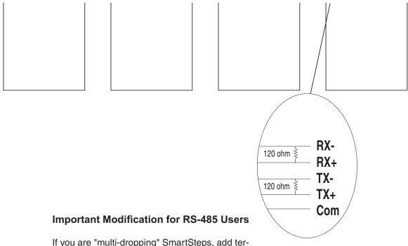
If you are "multi-dropping" SmartSteps, add termination resistors (120 ohms each) across RX and TX connections of the *last unit* as shown to the right.
