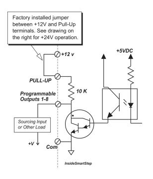
Max. sink current: 100 mA per output Total 350 mA available from 12VDC supply
