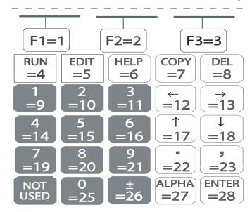
The following example shows how to use the keypad function keys as an operator interface.
