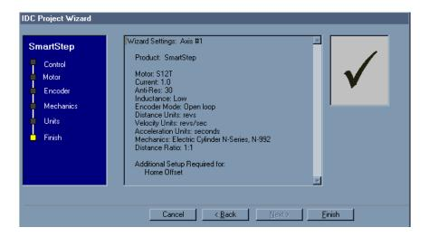
12. When you are satisfied with the setup of your system, click on **Finish**. Note that the Wizard Navigator now indicates that all axes and parameters have been configured.
