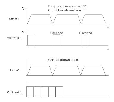
After the first pass through, the Loop command (LP) will wait at the GI command since subsequent GI moves must wait for the present move to finish.
