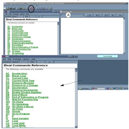
The drop down menu box (A) in the upper left hand corner shows the number and name of the currently active program, plus a list of up to 399 more programs. When the entire file is downloaded to the SmartStep, these program numbers correspond to the program numbers the controller uses for binary and BCD program selections.
