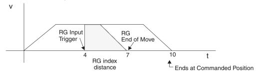
Accompanying the programmable Registration Command is the configurable Registration Input: G (also G in Serial Setup Commands). To configure a Registration input from the keypad, choose EDIT > SETUP > I/O > INPUTS. An input configured as a Registration Input will be designated by a G on the keypad input status display. The RG Command will only function if the corresponding input has been configured as a Registration Input (see note).
