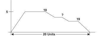
Using the DC formula and solving for DC<sub>n</sub>,  $DC_n = \frac{(|5-3|)(2.5)}{2} + 10 = 12.5$  therefore, the "?" must be greater than or equal to a position of 12.5 distance units. In addition to verifying the DC trigger position, it must also be verified that the DC? VE2.5 segment can be completed before the beginning of the move deceleration. Suppose the "?" was chosen to
