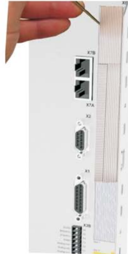
2 - Detach the film (at the perforations)
