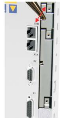
6 - Pull out the top plate
