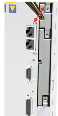
6 - Pull out the top plate
