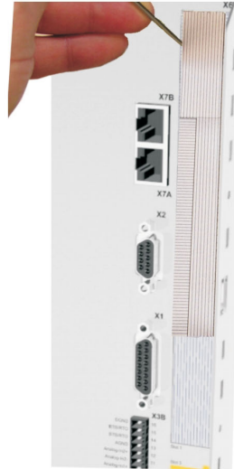
2 - Detach the film (at the perforations)
